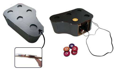
• RFID and button concept. Pushing the top surface allows switch to be actuated while allowing the PN532 to read RFID tags
